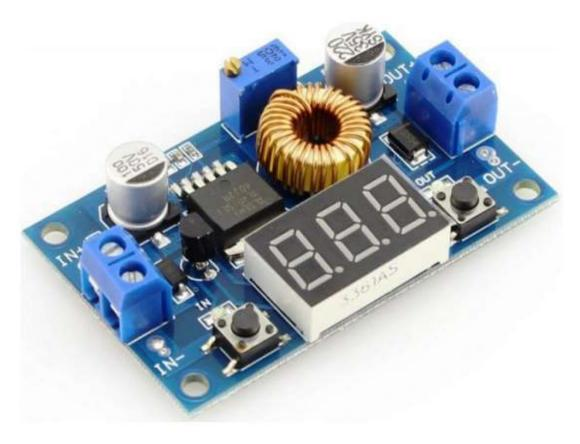
The module is available as a pre-populated board and requires zero soldering — it comes ready to go out of the box. Also, there's an extra heatsink for the XL4015 chip included with it. Major components in the module are showed in the following figure:
